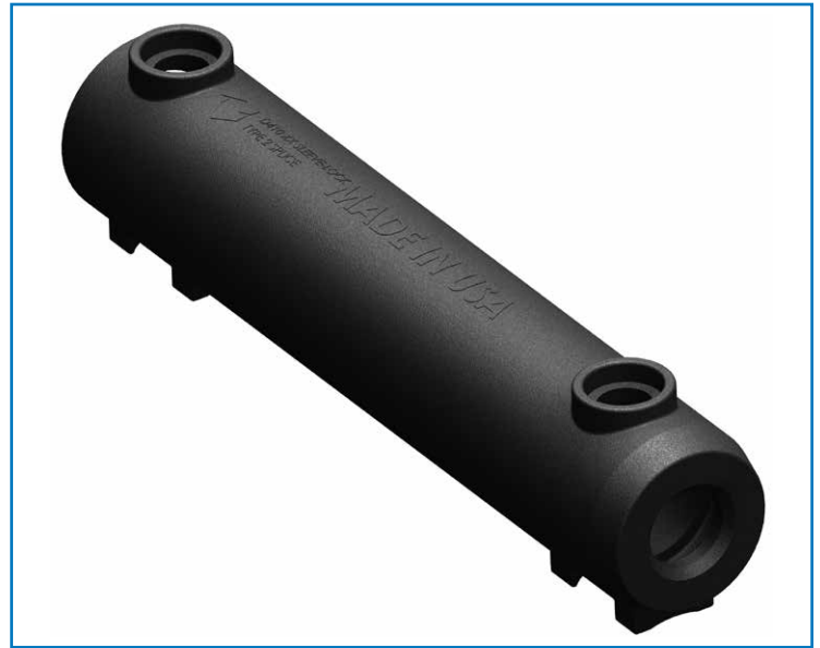
Grout is pumped into the Sleeve-Lock Grout Sleeve through tubes to lock rebar in place.
