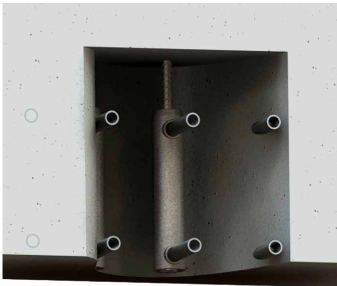
Once set fully in place, grout is injected into the embedded sleeve to create a strong connection.
