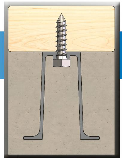
Note: The lag screw does not rotate independently of the cone, the T72 is one, assembled unit.
