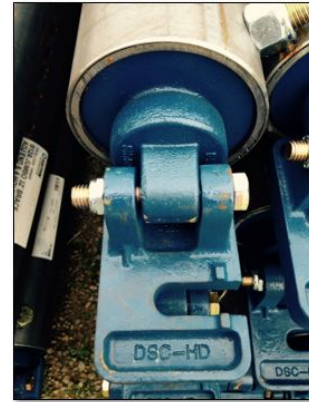
Photo #1: Swivel Assembly with Foot/Wall Plate. Rotate Plate out of way to access line of sight to pin (Note: Some versions have pin perpendicular to bolt and visible without moving plate)
