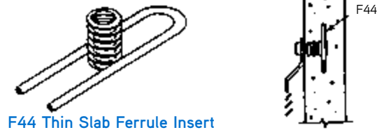
F44 Thin Slab Ferrule Insert
