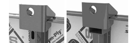
TOP TIE BRACKET AT VERTICAL CROSSMEMBER TOP TIE BRACKET AT TIE BOX TOP TIE BRACKET SAFE WORKING LOAD = 7,000 lbs. ● 2:1 SAFETY FACTOR
