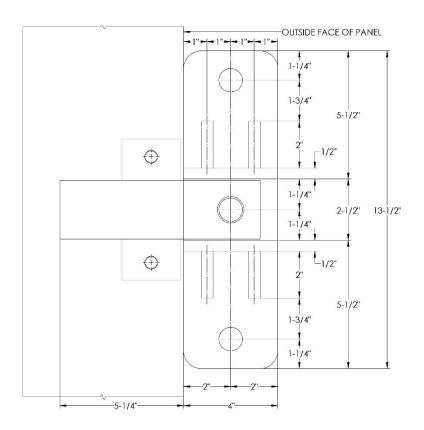
In-plane shear is resisted by the anchor insert bar bearing against the panel concrete and the shear anchor creating a moment couple.
