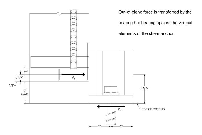
Steel Bearing design strength,  $\varphi R_n = \varphi(1.8)(F_y)(A_{pb})$
