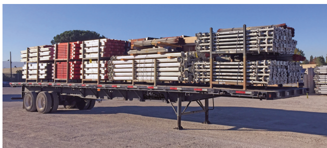
Typical 40' flatbed truck with 6,000 sq. ft. of shoring.
