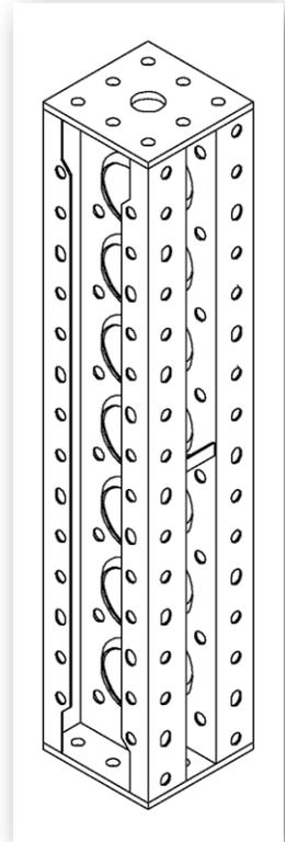
Symons Soldier beams permit bolting on all four flanges in addition to end and web bolt holes. The flange holes are a combination of holes and slots at 3" centers to provide dimensional adjustment and versatility.
