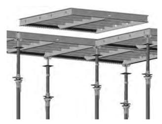
Insert panels into the DeckFast Bearing Supports from above the bearing supports.
