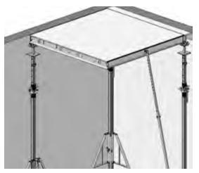
4. Put the Edge Support into position beneath the panel as shown, and plumb post shore.
