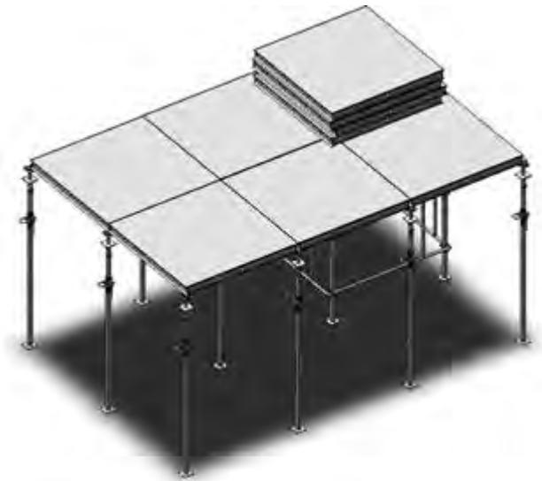
4. As the cantilevered panel reaches full length, lift the front end to capture the previously installed post supporting the adjacent panel and seat the rear corners properly in the rear post bearings.
