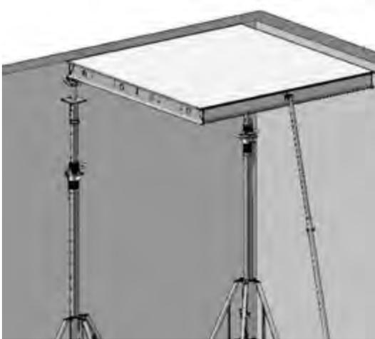
3. Swing the panel up with the DF Erection Rod and rotate it on the DeckFast Bearing until it rests firmly against the wall.
