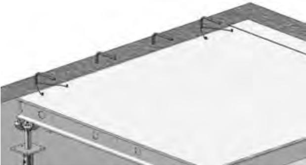
Panels may also be tied to rebar along the wall until the system is stabilized against the structure.
