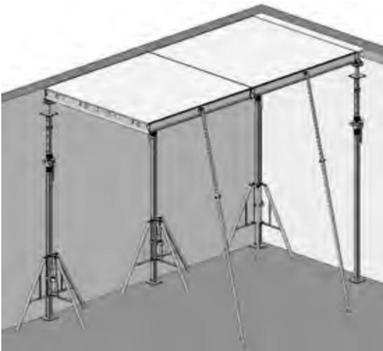
5. Raise the second panel the same as the first panel, and let it rest on a second Erection Rod.
