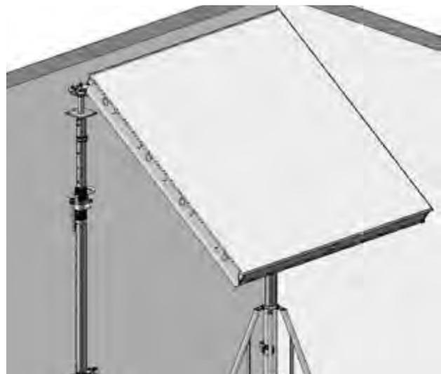
2. Hang the panel as shown. Make sure that the panel is hooked by the cams of both bearing devices. Hanging the panel requires two workers.
