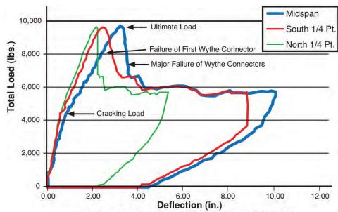
Note: All test panels were 6'-0" wide x 37'-0" long x 3"/2"/3" thick.
