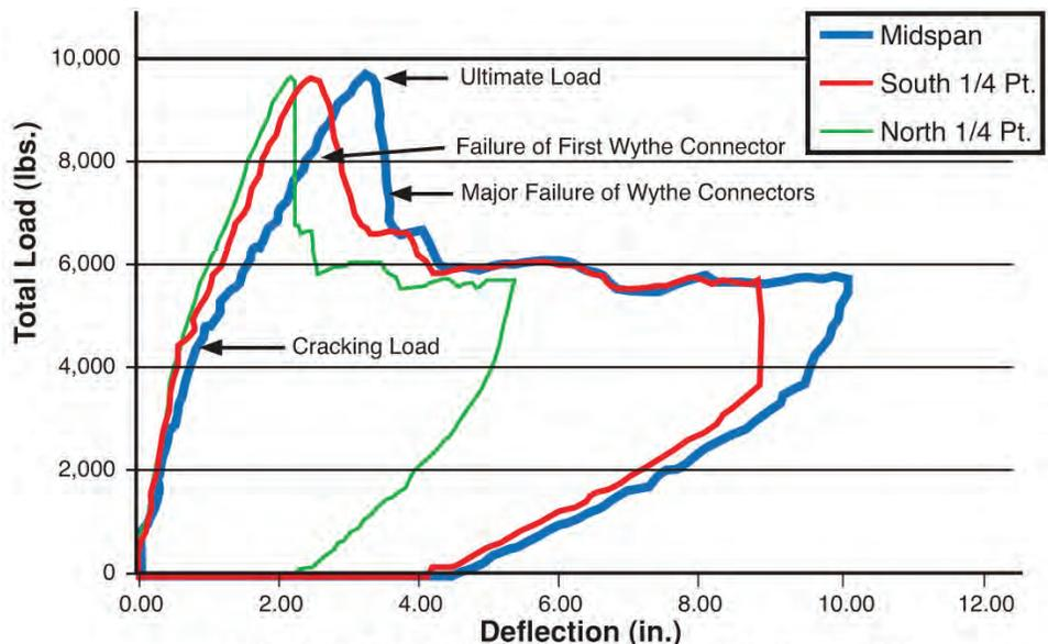
Note: All test panels were 6'-0" wide x 37'-0" long x 3 1/2"/3" thick.
