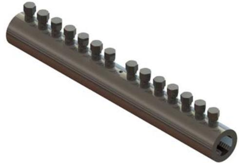
The thick-walled tube of the coupler is designed with lock shear bolts, serrated grip rails and center stop pins, providing a continuous path of mechanical reinforcing between two pieces of rebar. The coupler, compatible with Grade 75 and 80 rebar, is available for sizes #3 through #18. In addition, the coupler does not require a contractor to hire a third party as no bar end preparation is needed, ultimately saving time and money on the jobsite.
